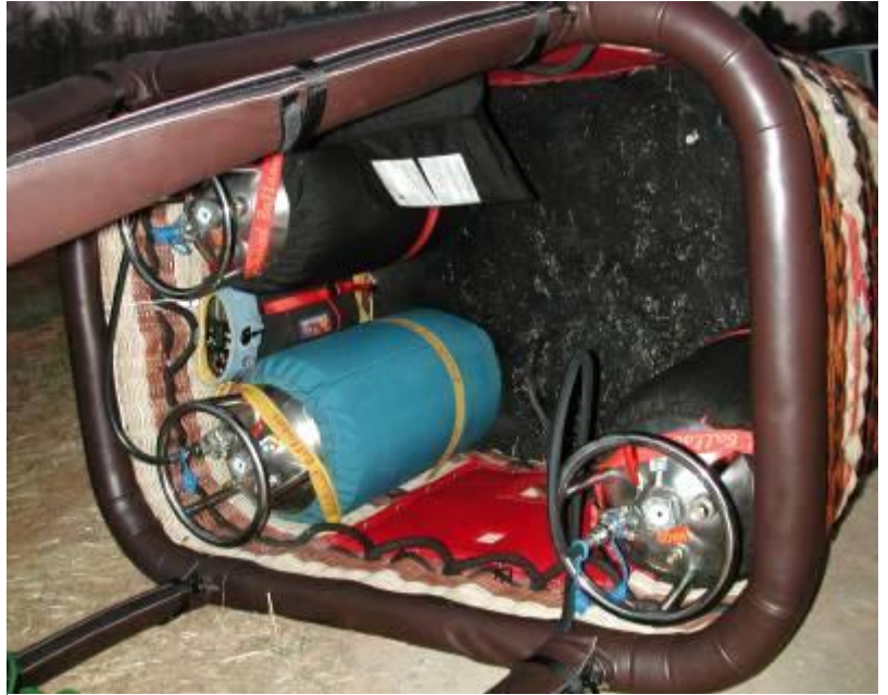
The basket holds the passengers, propane tanks and navigation equipment.
